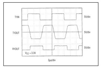
Figure 11. Loopback Test Result at 250kbps
