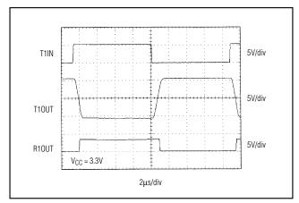
Figure 10. Loopback Test Result at 120kbps
