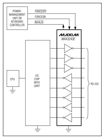
Figure 1. Interface Under Control of PMU
