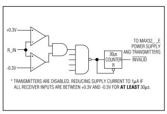
Figure 3a. MAX32\_\_E Entering 1µA Supply Mode via AutoShutdown
