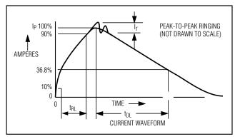
Figure 6b. Human Body Model Current Waveform
