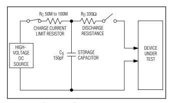
Figure 7a. IEC1000-4-2 ESD Test Model
