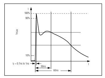
Figure 7b. IEC1000-4-2 ESD Generator Current Waveform
