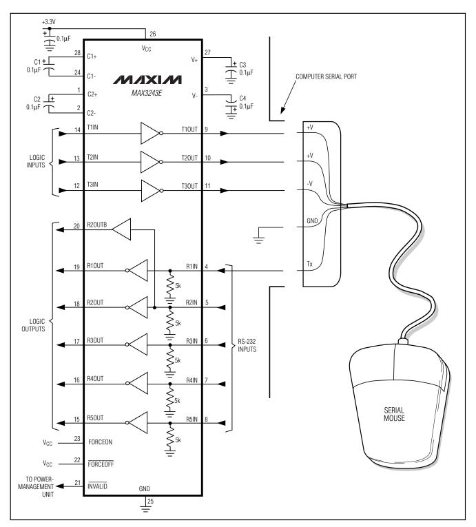
Figure 12b. Mouse Driver Test Circuit
