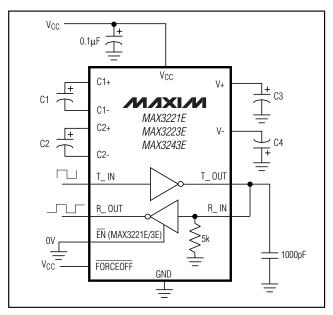
Figure 9. Loopback Test Circuit
