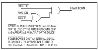
Figure 3c. MAX32\_ \_E AutoShutdown Logic
